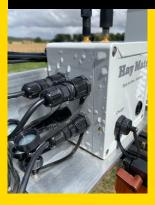
One base unit allows up to 4 sensors plugged into it
